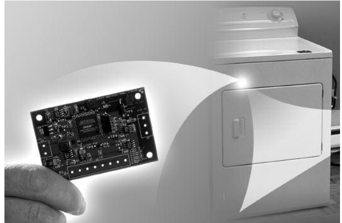
Graphic depicts chip developed by Pacific Northwest National Laboratory that gives home appliances on-board intelligence to respond to grid conditions.
